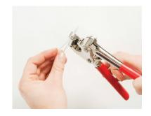
2 Insert the Alucast seal into the Seal Nipper and press the pliers firmly together.
