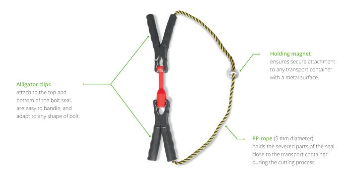
1 Attach magnet to metal surface of container or truck door. Affix one alligator clip of the Bednorz K Protector to the top of the bolt seal and one to the bottom.
