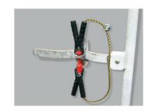
3 The bolt seal can now be cut safely with bolt cutters.
