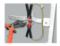
4 The fragments of the bolt seal remain reliably secured by the two alligator clips.
