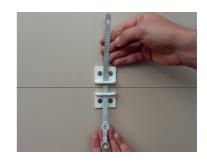
2 Bend the top of the strap downwards and position the pin in the oval slot.
