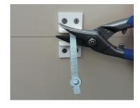
At least 5mm of unmarked strap head should be visible between the seal head and the embossed section of the strap. The end of the strap should also be clearly visible from the side of the sealhead and should move freely within the oval slot.
