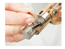
Feed the wire or string through the apertures of the item to be sealed (not shown). Tie a simple knot where the seal should be fastened and place the jaws of the Coding Nipper either side of it.
