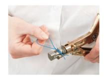
4 Squeeze the levers of the Coding Nipper together. This winds the lower, serrated part of the roll tag tightly around the wire or string. If customised dies are used, an initial or logo is simultaneously embossed onto the plain front.
