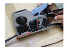
When the required tension is achieved, push the button at the end of the tension lever, and continue to rock the lever back and forth until there is some resistance. This means that the ends of the strapping are now connected by the strapping seal. Firmly press down the tension lever to cut the strap. The tool can now be removed.
