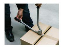
**7** Press the lever arm down to punch a slot through the strapping seal.
