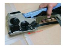
4 Push the other end of the strapping through the loaded strapping seal and then through the cross-head holder. Tighten the strapping around the package by rocking the lever back and forth.
