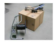
2 To tightly wrap the package with strapping, load a strapping seal into the One Hand Strapping Tool
