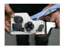
3 Slide one end of the strapping from the back of the mechanism to the front, threading it through the loaded strapping seal. Then firmly press down the tension lever.
