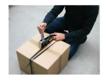
6 Slide the mouth of the Slot Punch Pliers fully over the strapping seal.
